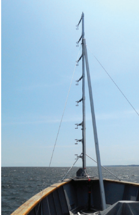
FIGURE 5. Bow anemometer array. Reference anemometer is third from bottom.
