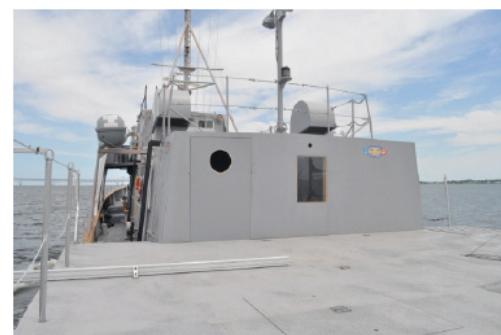
FIGURE 3. Detail of YP676 flight deck and hangar-like structure.
